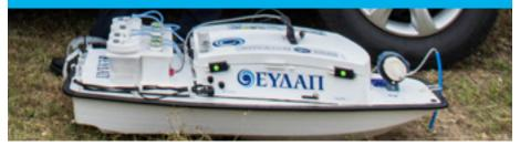
**In 2021** inspections with autonomous vessels continued in all EYDAP's reservoirs and **more than 250,000 readings** were collected along a total of more than 90 kilometres around the Reservoirs.
